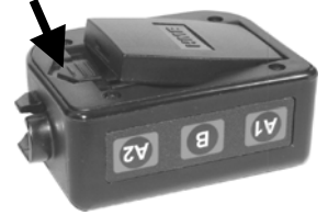
Figure 6. Communicator battery-release latch
